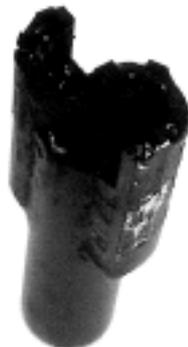
It doesn't collapse bore-hole easily. So, especially, it is effective for mudstone.
