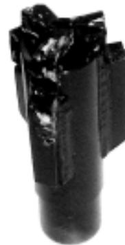
It is suitable for soft-rock stratum of mudstone and tuff. One piece of the blades expand to the center of water supply-hole, so there is no clogging of core.
